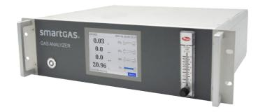
The ANAREX  $SF_6$  analyzer of smartGAS is a high-performance solution for the leakage detection in high voltage application. It convinces with its highly accurate and stable measurement performance as well as its customer-friendly interfacing via touch screen along with a simple sensor calibration.
